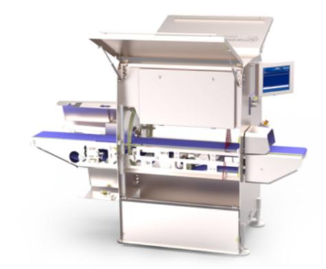
The Marelec PORTIO 9 is our step-in model for high-precision portion cutting, designed for fish and poultry processing. The "9" refers to its 9-inch belt width, making it a compact yet powerful solution for food processors.
