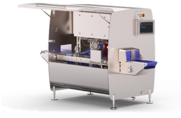
In addition to its top-mounted camera, the PORTIO 12 can be operated with two lateral cameras to create more rounded products - an effect further enhanced by a feature that can alter the angle of the knife from the 0° (vertical) position, to 30° or 45°. Cutting at an angle gives a natural look to sliced portions or creates a bigger plate coverage.
