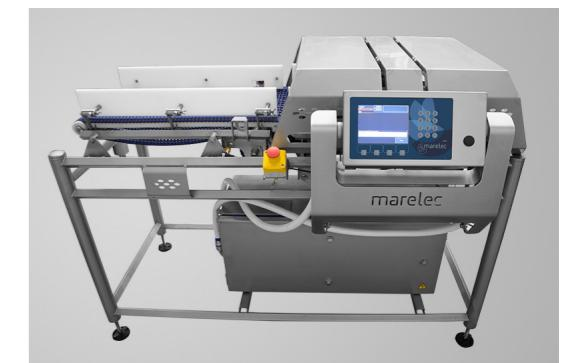
The same result can be obtained with a density scale. This density scale can be used with reverse weighing, meaning the operator can weigh a crate with several primals and feed them one by one. This will allow the density scale to communicate the weight of each individual product to the Portio B which will correct the density automatically.
