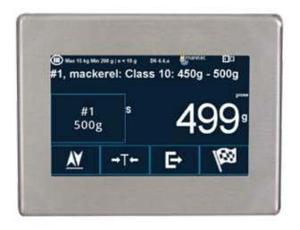
This mode allows the operator to define a set of weight ranges on the scale (operator can change species and classes on the MARELEC D6B which can be labelled. The scale will then proceed to assign a defined range to any current weight whenever the readout is stable.
