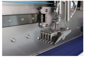
While the gripper ensures that the primals don't move backwards, the topholder prevents products from moving sideways on the feeding section. The combination of gripper and top holder will guarantee accurate fixed-weight cuts with high cutting quality, ready to be presented in a retail package.
